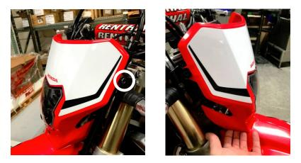
2. While facing the headlight, look down the back of the faceplate and locate the cord routing clip on the left (Circled in the image below). Using the needle-nose pliers, squeeze the prongs together until the clip is free from the headlight.
