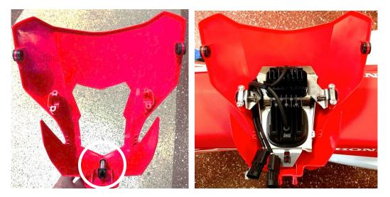
6. On the OEM headlight, remove the retaining clip mount from step 2 with the T20H Torx bit (Circled on left image below). Remove the rectangular module mount as well (not pictured on left, arrow shows location). Using the provided hardware and 4mm Allen wrench, reorient both mounts and attach them referencing the image on the right below.
