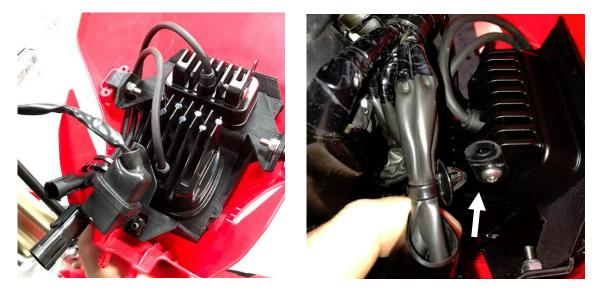
8. Push the faceplate pins down into the fender until they seat completely. Replace the two 10mm hex head bolts from step 1 and tighten.
